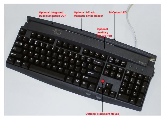
The Access ATB422/423 keyboard is a compact standard Windows layout keyboard with integrated electronics to capture data from a variety of sources.
